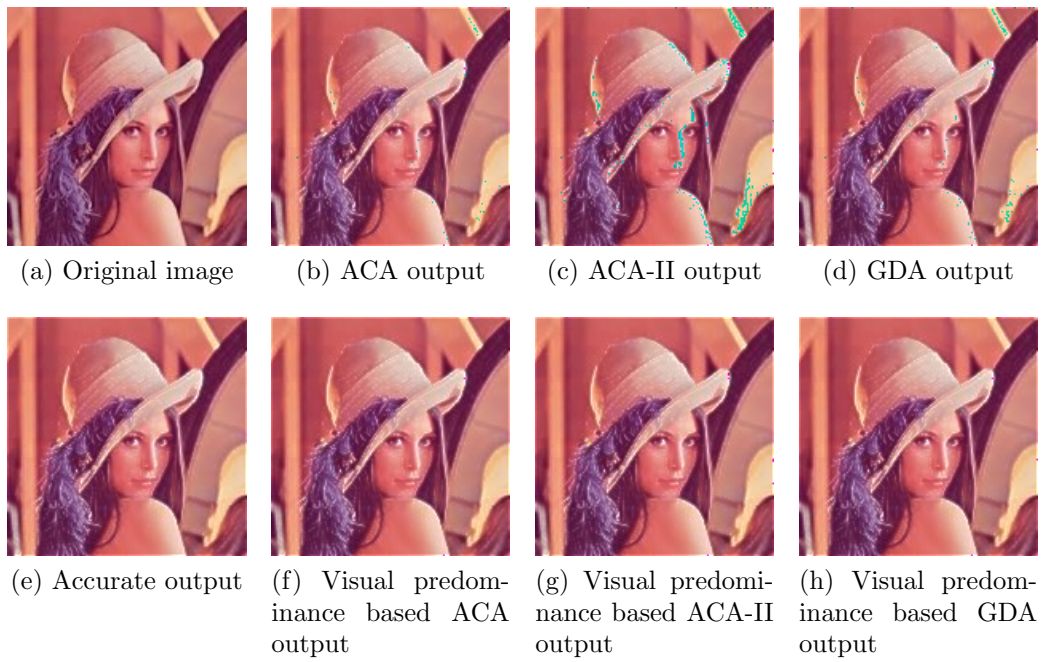
Figure 5: Unsharp masking of an image accurately and using approximate adders.
